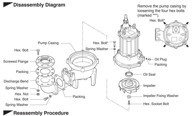
Observe the precautions given below and reassemble the unit in the reverse order of disassembly.
