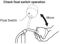
**Note:** Allow the pump to operate a minimum of 2 seconds for each trial operation. The trial operation must be completed within 1 minute.
