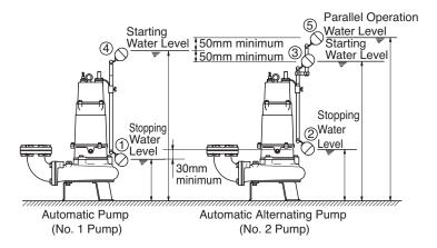
Adjusting the start float to set the starting water level as desired:
