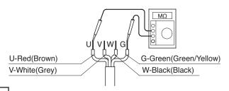
Insulation resistance reference value = 20M  $\Omega$  minimum
