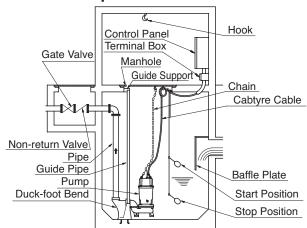
(1) When transporting or installing the pump, do not kink the cabtyre cable or use it in place of a rope.
