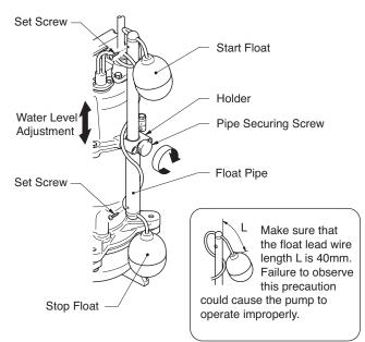
To change the operating water level on an automatic alternating model, perform the setting by referring to the diagram on the right.
