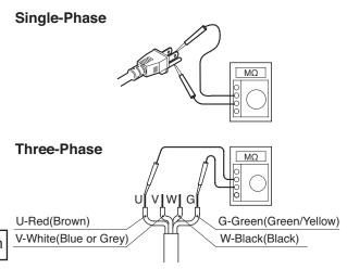
**Note:** The insulation resistance reference value of 20M  $\Omega$  minimum is based on a new or repaired pump. For reference values of a pump that has already been put into operation, refer to "7. Maintenance and Inspection" of
