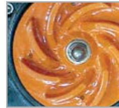
Tsurumi Impeller polished, not worn by abrasive material.
