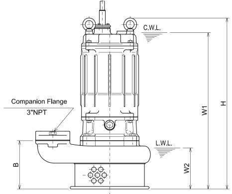
C.W.L. :Continuous running Water Level L.W.L. :Lowest running Water Level
