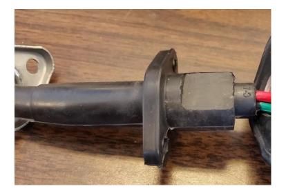
4. Pull the cable gland through the relay unit so the flat part rests against the wires from the relay unit
