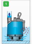
Pump continues to run while e-probe remains submerged.
